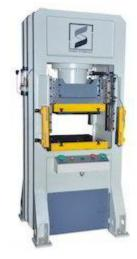
Pump 210 kg/cm2 - 90 l/min Motor 200v 50H2 - 30 kwx6 P Oil – 600 L
