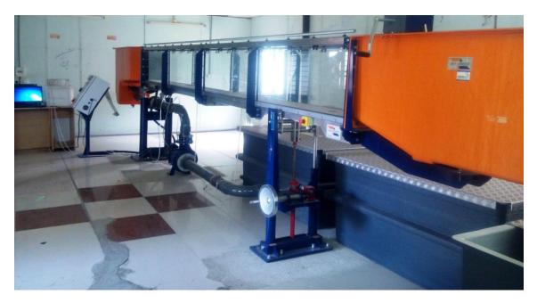
**Application:** The flow channel or flume is one of the most important tools available to the hydraulics engineer or civil engineer whether engaged in teaching researching solutions to practical problems. Many applications in fluid mechanics are associated the flow of water through an open channel where the water has a free surface that is exposed to the air at atmospheric pressure.
