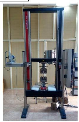
**Applications:** Tension and compression tests at room temperature and high temperatures as well as bending (3 point) at room temperature.
