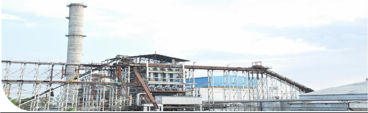
Fig: Conveying system to transport material from storage unit to Furnace section
