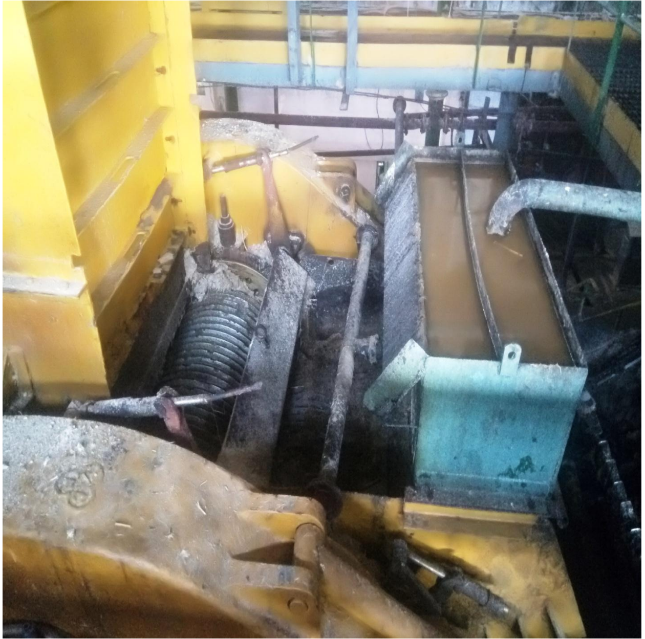
Fig: Roll crushers to extract Juice from sugar cane
